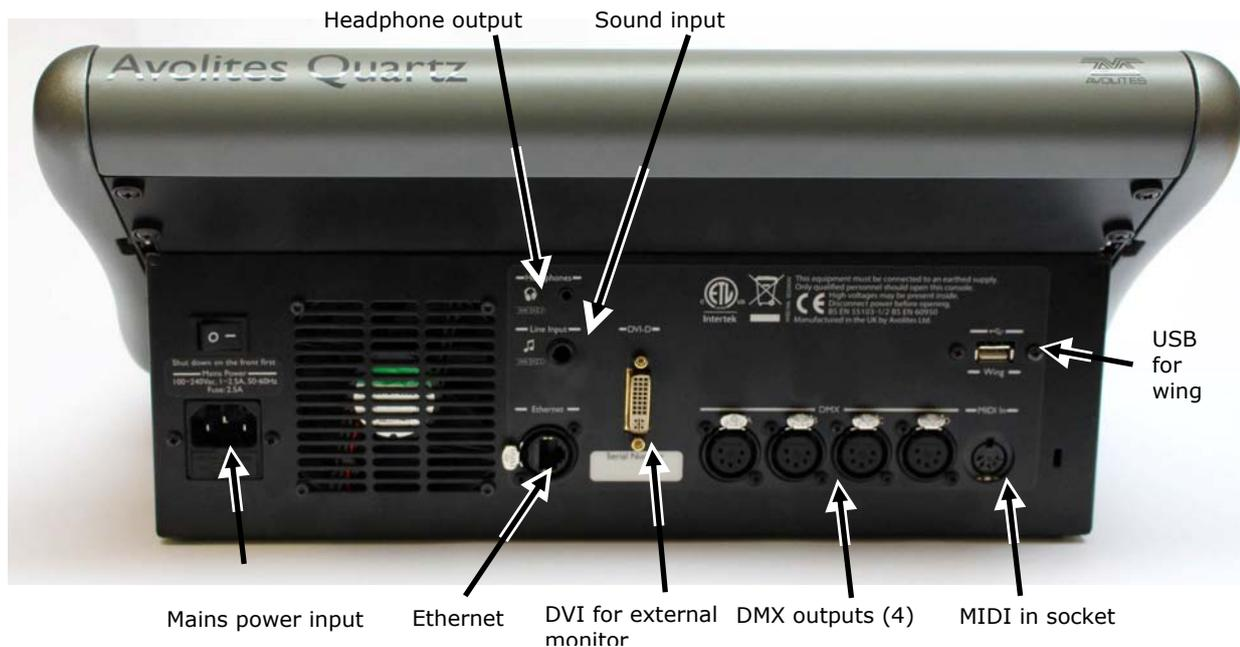
All the connections are on the rear panel. Most are self-explanatory. The power switch on the rear panel is an isolator for the power supply and should not be used to turn the console off. Use the switch on the front panel to turn the console on and off.
